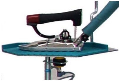
Fig. 19 Example 9: Safety Iron Rest
