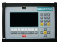
Fig. 4 INDUMAT 07 - Graphical user interface with detailed info and error messages
